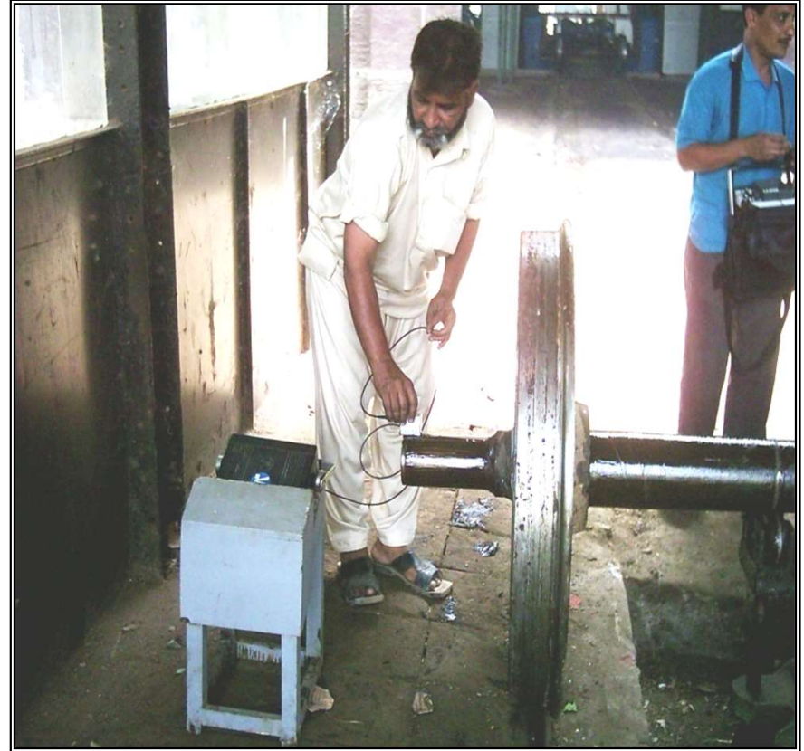
Ultrasonic Testing Shop
